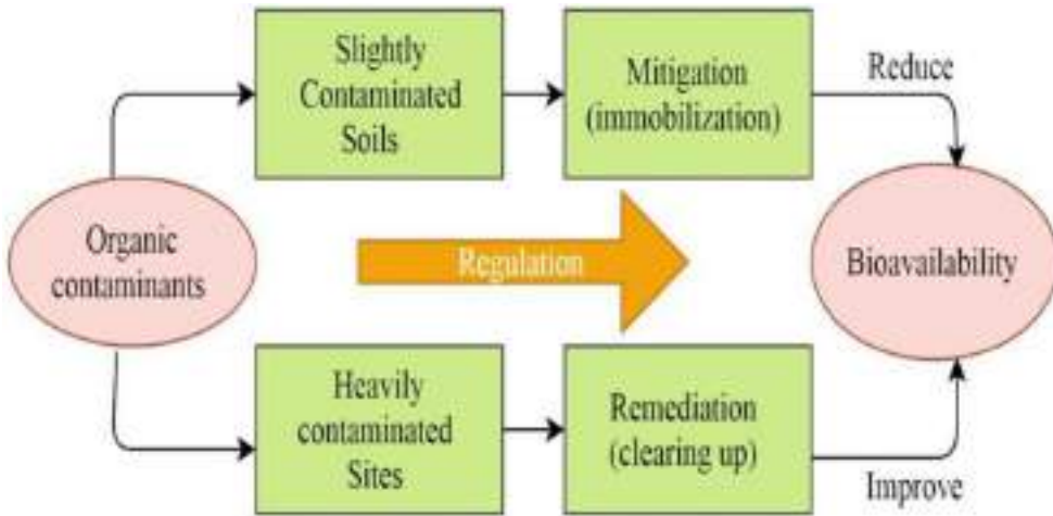
Figure 6. Strategies of mitigation and remediation for slightly and heavily contaminated soil.
