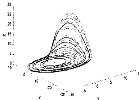
Fig.4 Rossler attractor with a=0.2 , b=0.2 and c=5.7
